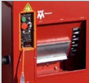
Manual material adjustment through sieve and slide gate
